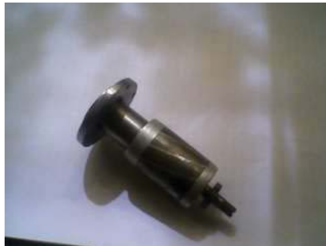
Photo. 2. Flexible squirrel cage rotor.
